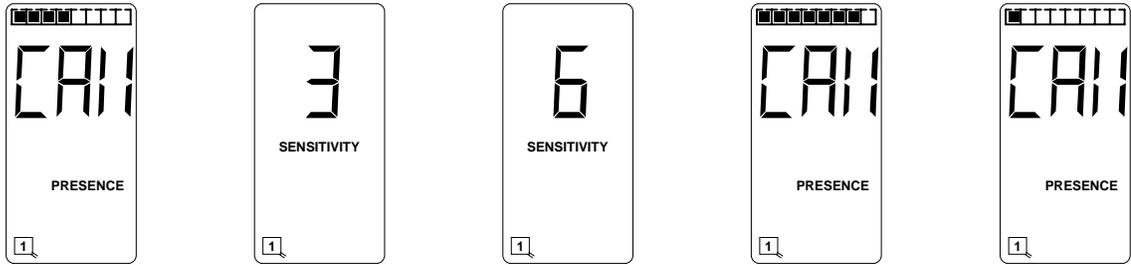
**Step 1:** Observe a single standard automobile in the loop zone. Note the number of segments displayed on the bargraph. **(4)**
