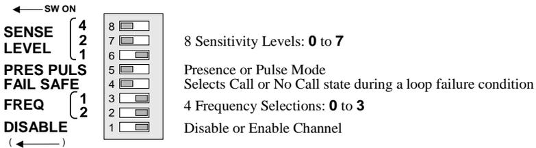
Front Panel Eight-position DIP Switch Module
