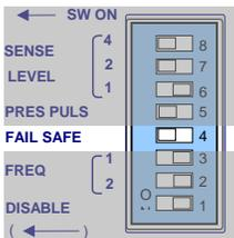
**Fail-Safe / Fail-Secure:** DIP switch 4 sets the default state of the channel's output when a loop failure condition exists on the loop network connected to the channel. One of two output states, shown in the table below, can be selected during a loop failure condition.
