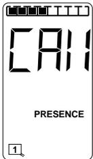
**Step 1:** Observe a single standard automobile in the loop zone. Note the number of segments displayed on the bar graph. (4)
