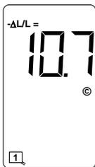
**STATE**.....% Loop Inductance Change (- $\Delta$ L/L) Display (Option 1 ON).
