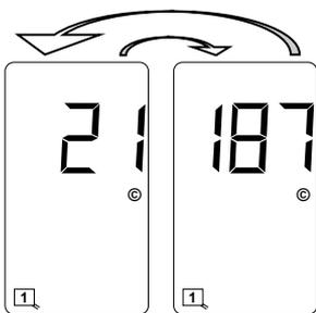
**STATE**.....Accumulated Vehicle Count Display (Option 2.0 ON).
