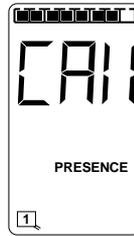
**Step 4:** Verify that a single standard automobile causes the bargraph to move seven segments.
