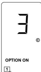
**PARAMETER** .....Option 3 (Relay B Buzzer).
