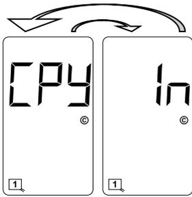
Parameters stored on the motherboard mounted EEPROM do not match those stored on the internal EEPROM. Pressing the **FUNC** pushbutton will accept the parameters stored on the internal EEPROM and store them on the motherboard mounted EEPROM, i.e. copy the internal EEPROM parameters to the motherboard mounted EEPROM.
