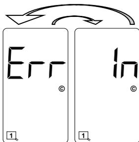
**Internal EEPROM Error.** The display will toggle between the two screens shown with a 50% duty cycle. This is an indication that the data stored on the internal EEPROM is corrupt. Press the **FUNC** pushbutton to copy the reference data stored on the motherboard mounted EEPROM to the internal EEPROM. If the error message does not clear, the internal EEPROM is defective. Return the detector to the factory for servicing.
