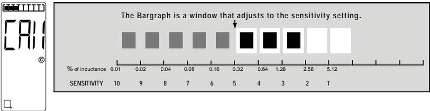
The bargraph below has the same vehicle in the loop zone causing the same inductance change as above. Because the sensitivity setting was increased to Level 8, six segments are now displayed. If the bargraph displays 5 or 6 segments for a vehicle in the loop, the sensitivity has been set to the proper range.
