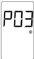
Upon application of power, the LCD screen will show the detector model letter and firmware version, in this case, Model P-1400 firmware version 3. This screen will be displayed for two seconds.
