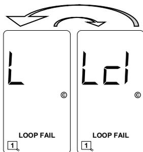
Loop Check Failure Indication
