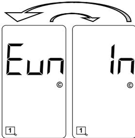
**Uninitialized Internal EEPROM.** The display will toggle between the two screens shown with a 50% duty cycle. This is an indication that the internal EEPROM is uninitialized. To correct this problem, press the **FUNC** pushbutton. If the error message does not clear, the internal EEPROM is defective. Return the detector to the factory for servicing.
