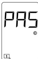
The Loop Check feature is enabled whenever the Loop Check Timer for a specific loop input is set to a value between 1 and 255 minutes. When the Loop Check Timer has timed out, the detector will automatically short the check loop to simulate vehicle detection. If the percentage of inductance change is greater than or equal to -0.04%  $\Delta L/L$ , and the channel on which the current loop check test is selected and being viewed on the LCD, the display will show **PAS**.
