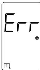
**Detection Reference Error.** This is an indication that the internal EEPROM and the motherboard mounted EEPROM detection reference values do not match. Press the **FUNC** pushbutton to clear the error message.
