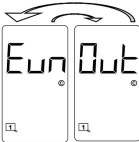
**Uninitialized Motherboard Mounted EEPROM.** The display will toggle between the two screens shown with a 50% duty cycle. This is an indication that the motherboard mounted EEPROM is uninitialized. To correct this problem, press the **FUNC** pushbutton. If the error message does not clear, the motherboard mounted EEPROM is defective. Return the detector to the factory for servicing.
