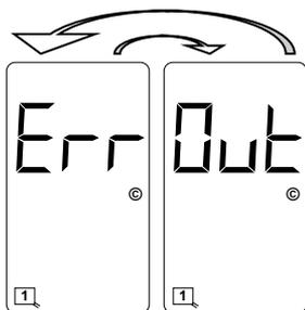
**Motherboard Mounted EEPROM Error.** The display will toggle between the two screens shown with a 50% duty cycle. This is an indication that the data stored on the motherboard mounted EEPROM is corrupt. Press the **FUNC** pushbutton to copy the reference data stored on the internal EEPROM to the motherboard mounted EEPROM. If the error message does not clear, the motherboard mounted EEPROM is defective. Return the detector to the factory for servicing.
