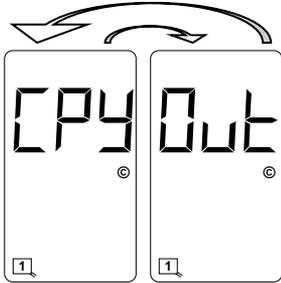
Parameters stored on the motherboard mounted EEPROM do not match those stored on the internal EEPROM. Pressing the **FUNC** pushbutton will accept the parameters stored on the motherboard mounted EEPROM and store them on the internal EEPROM, i.e. copy the motherboard mounted EEPROM parameters to the internal EEPROM.
