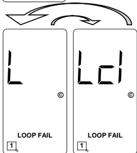
If the check loop verification process continues for the entire 55 second period and no action has been taken to connect or restore the check loops causing the check loop verification, the LCD screen will toggle between the two screens shown with a 50% duty cycle.
