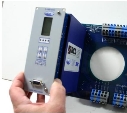
Step 5: Remove the microcontroller, located near the upper right corner of the PC board. To avoid damaging the microcontroller socket, it is strongly recommended that a tool designed for this purpose is used.
