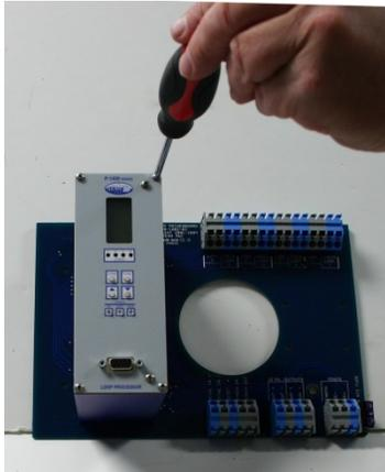
Step 3: Insert the end of the small, flat bladed screwdriver between the front panel and the detector housing. Carefully twist the screwdriver to pry the front panel away from the detector housing. To avoid damaging the detector PC board, do not insert the screwdriver more than 0.125 inch.
