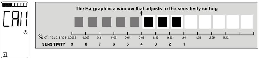
The bargraph, below, has the same vehicle in the loop zone causing the same inductance change as above. Since the sensitivity setting was increased to Level 7, six segments are now displayed. If the bargraph displays 5 or 6 segments for a vehicle in the loop and motorcycles are not a concern, the sensitivity has been set to the proper
