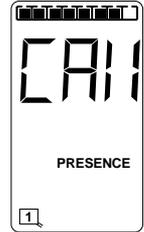
**Step 1:** Observe a single standard automobile in the loop zone. Note the number of segments displayed on the bargraph. (4)
