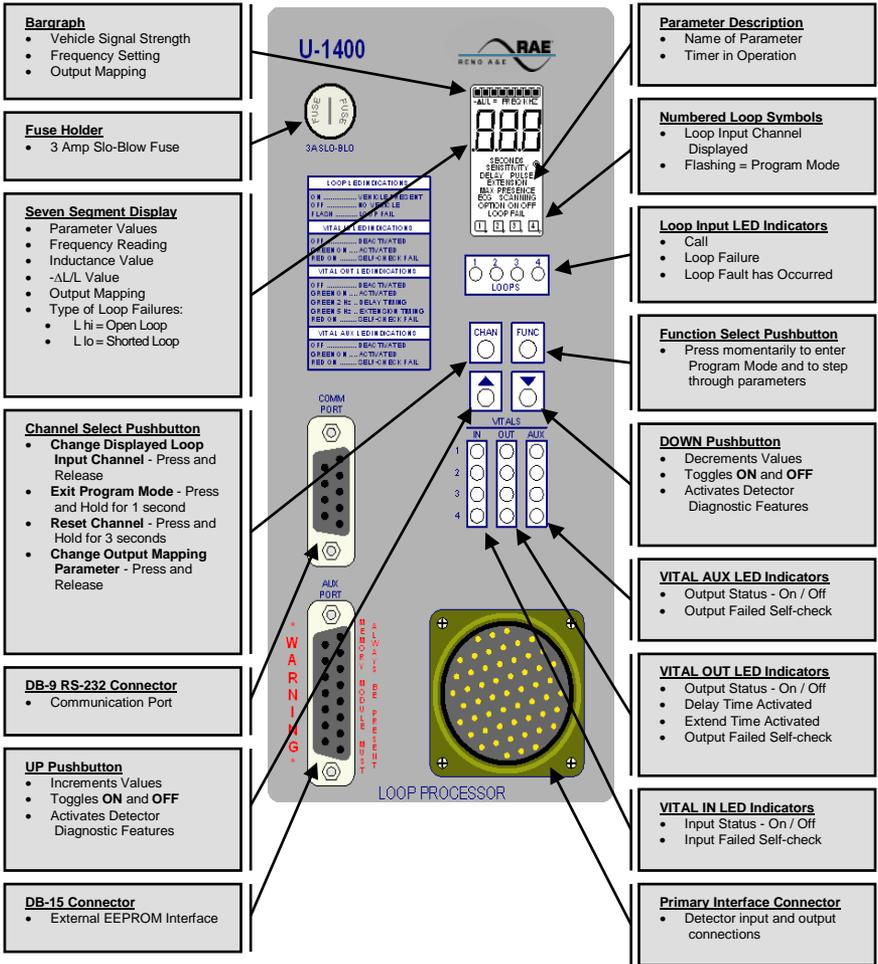
**NOTES:** The LCD backlighting illuminates whenever any pushbutton is pressed. Backlighting will extinguish 15 minutes after the last pushbutton press.
