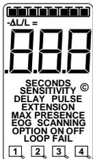
STATE .....LCD Display Test.
