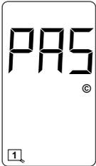
The detector will next confirm the state of the check loops connected to it. If all four check loops are connected and are intact, the LCD screen will display an indication of the successful completion of the check loop verification. This screen will flash twice.
