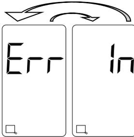
**Internal EEPROM Error.** The display will toggle between the two screens shown with a 50% duty cycle. This is an indication that the data stored on the internal EEPROM is corrupt. Press the **FUNC** pushbutton to copy the reference data stored on the external EEPROM memory module to the internal EEPROM. If the error message does not clear, the internal EEPROM is defective. Return the detector to the factory for servicing.
