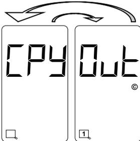
Parameters stored on the external EEPROM memory module do not match those stored on the internal EEPROM. Pressing the **FUNC** pushbutton will accept the parameters stored on the external EEPROM memory module and store them on the internal EEPROM, i.e. copy the external EEPROM memory module parameters to the internal EEPROM.
