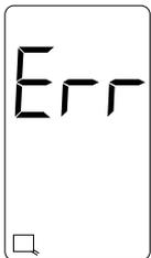
**Detection Reference Error.** This is an indication that the internal EEPROM and the external EEPROM memory module detection reference values do not match. Press the **FUNC** pushbutton to clear the error message.
