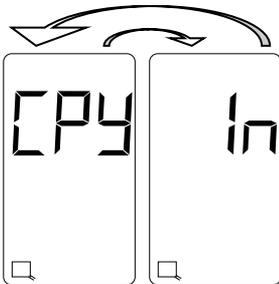
Parameters stored on the external EEPROM memory module do not match those stored on the internal EEPROM. Pressing the **FUNC** pushbutton will accept the parameters stored on the internal EEPROM and store them on the external EEPROM memory module, i.e. copy the internal EEPROM parameters to the external EEPROM memory module.
