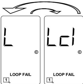
If the check loop verification process continues for the entire 55 second period and no action has been taken to connect or restore the check loops causing the check loop verification, the LCD screen will toggle between the two screens shown with a 50% duty cycle.
