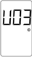
Upon application of power, the LCD screen will show the detector model letter and firmware version, in this case, Model U-1400 firmware version 3. This screen will be displayed for two seconds.
